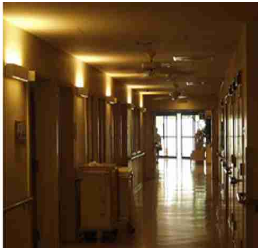
Figure II: An example of lighting problems a) extremely low light levels, b) uneven lighting, and c) glare from doors at the end of the corridor.
